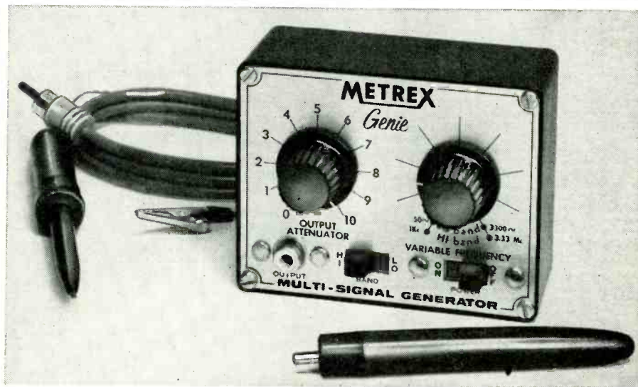
This 3½ x 1½-inch instrument is a complete transmitting station.
