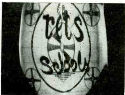
Fig. 2—Long narrow raster with a heavy drive line down the center was caused by the screen-grid resistor on the horizontal output tube increasing in value.
