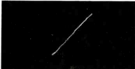
Fig. 3 —Scope connected to check power in resistive load R_L (a) produces the straightline pattern (b) that shows 100% real power in the load.
